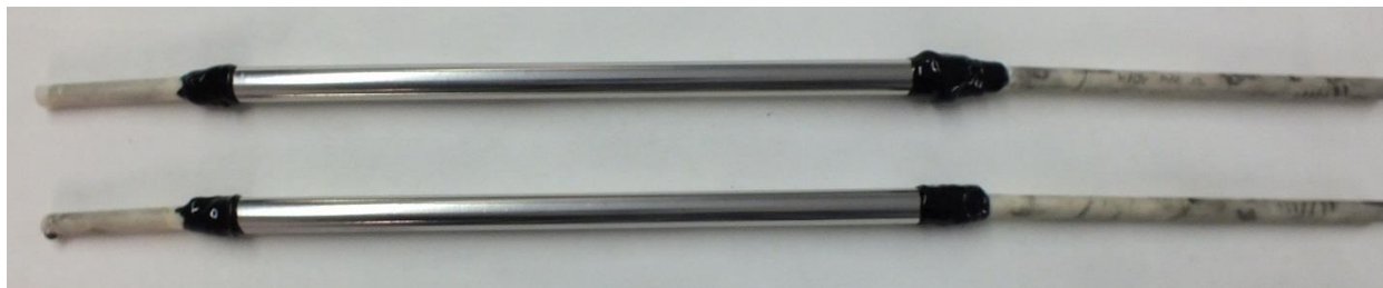
Thin film Pd-alloy (< 5 µm) supported membranes
