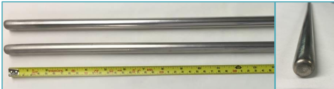
2 nd generation thin film Pd-alloy supported membranes
