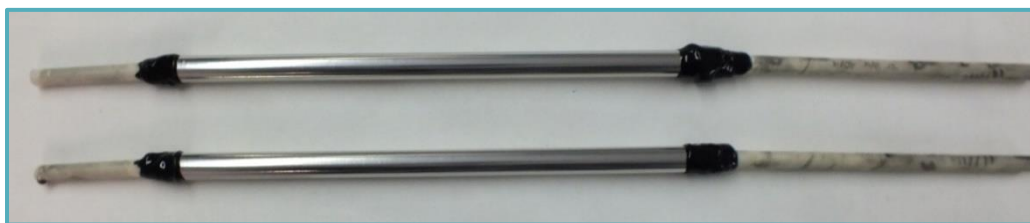
1 st generation thin film Pd-alloy (< 5 \mu\text{m} ) supported membranes
