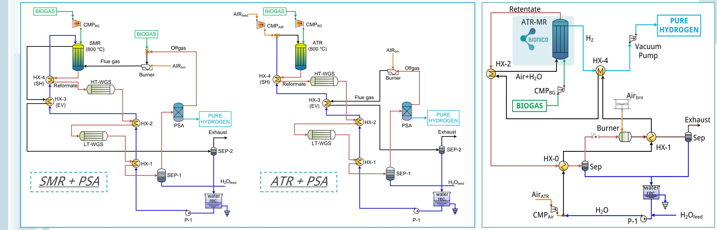
The ceramic supported membranes are integrated in a autothermal reforming reactor (ATR-MR). The investigated layout adopt a vacuum pump in order to reduce the hydrogen partial pressure on the permeate side. Thanks to the choice of the vacuum pump, instead of a sweep gas, the total required membrane area will be lower. The reactor operating temperature for the reference case is assumed up to 550-600 °C, in order to preserve the membranes lifetime.
